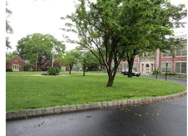
Two rain gardens can be installed in the front and back of the building in the turfgrass areas to help infiltrate the water from the nearby downspouts. A preliminary soil assessment suggests that the soils have suitable drainage characteristics for green infrastructure.
